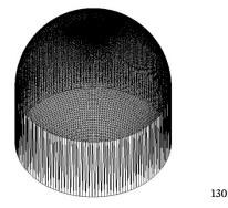
.stl files can be prepared in plain ASCII text, which is easier for humans to read but more storage-intensive than the more compact "binary" format, which is expressed in ones and zeroes.<sup>131</sup> An ASCII .stl example of the simplest possible polygon is given below (it is unrelated to the illustrations above). For each triangular surface, the file describes a set of vertices as well as a "normal," a vector that (perhaps redundantly) describes which face of the triangle
